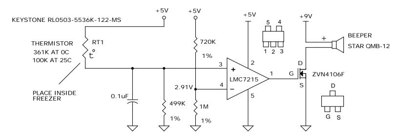
ACTIVATES THE BEEPER WHEN THE INSIDE FREEZER TEMPERATURE IS ABOVE ZERO DEGREES C OR 32 DEGREES F.
