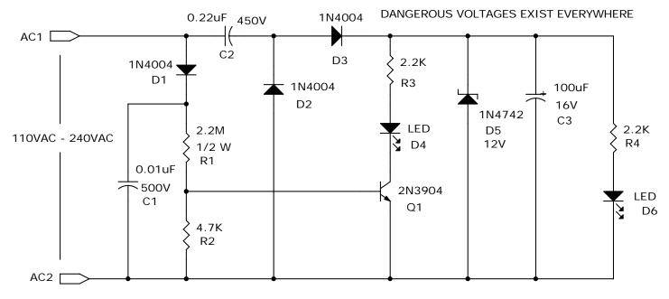
D6 TURNS ON WITH 110VAC D4 AND D6 TURN ON WITH 220VAC
