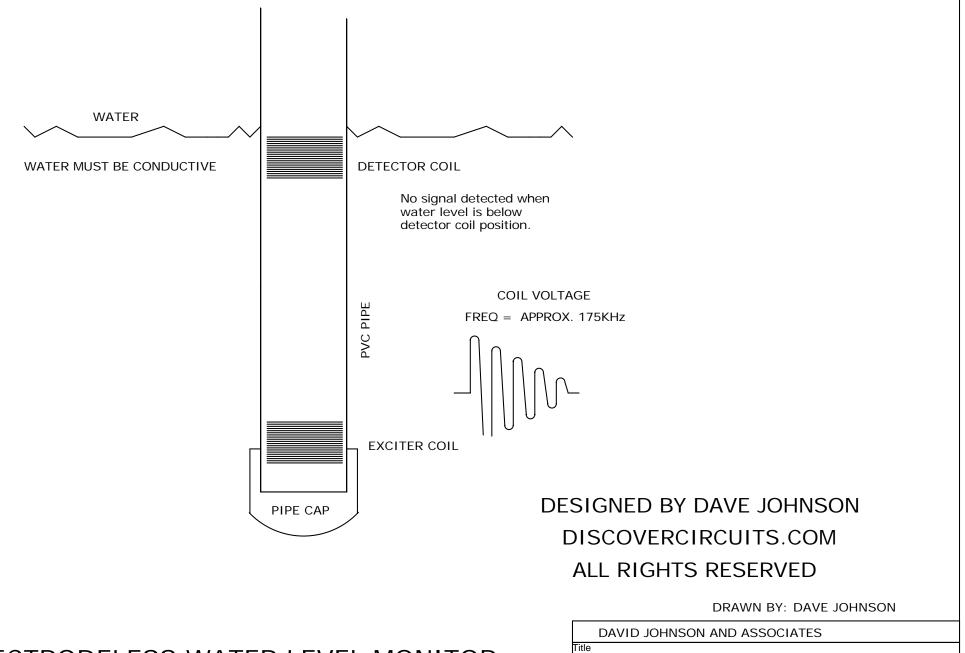
**ELECTRODELESS WATER LEVEL MONITOR**
