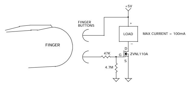
ELECTRICAL CONDUCTION THROUGH FINGER TURNS ON THE MOSFET
