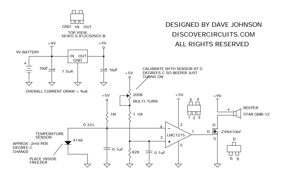
ACTIVATES THE BEEPER WHEN THE INSIDE FREEZER TEMPERATURE IS ABOVE ZERO DEGREES C OR 32 DEGREES F.
