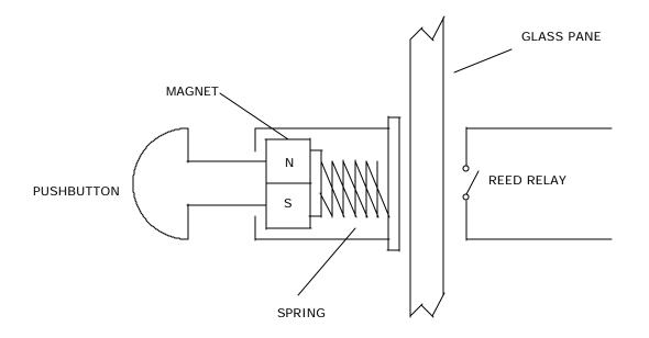
PUSHBUTTON MOVES MAGNET CLOSE TO GLASS MAGNET THEN ACTIVATES REED SWITCH
