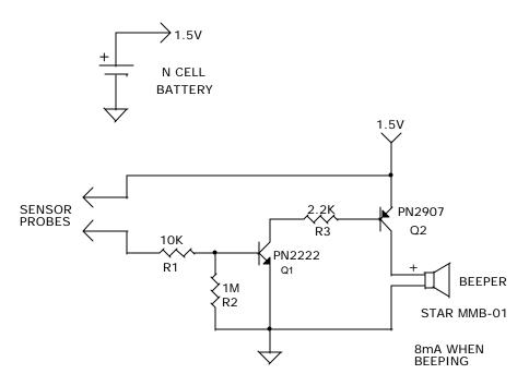
CURRENT CONDUCTION THROUGH WATER TRIGGERS ALARM BEEPER
