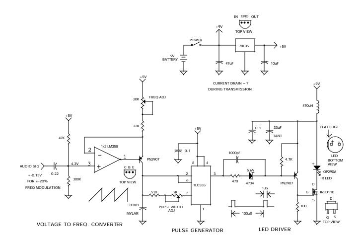
OPTICAL THROUGH THE AIR TRANSMITTER
