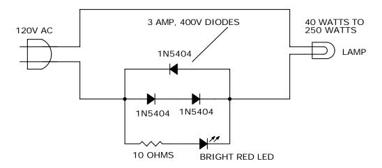
LED LIGHTS WHEN LAMP IS DRAWING CURRENT
