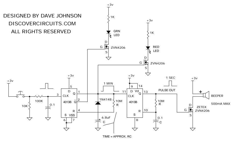
Pushbutton triggers short 1 second beep. Beep can't be activated again until after 1 minute timer ends.
