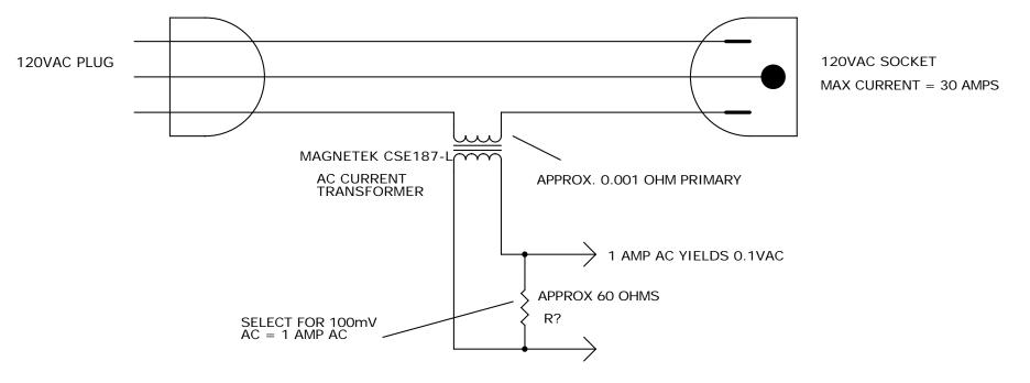
CALIBRATE WITH 100 OHM 100 WATT LOAD AND AC VOLTAGE SET AT 100VAC
