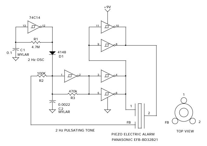
BEEPING CURRENT DRAIN = 12mA AT 9V SOUND LEVEL = 110dB AT 12" AT 9V
