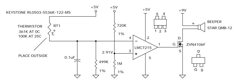
ACTIVATES THE BEEPER WHEN AIR TEMPERATURE IS BELOW ZERO DEGREES C OR 32 DEGREES F.
