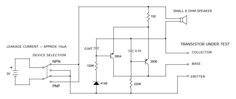
CIRCUIT IS AN OSCILLATOR THAT PRODUCES A TONE IN THE SPEAKER WHEN THE TRANSISTOR TESTS GOOD
